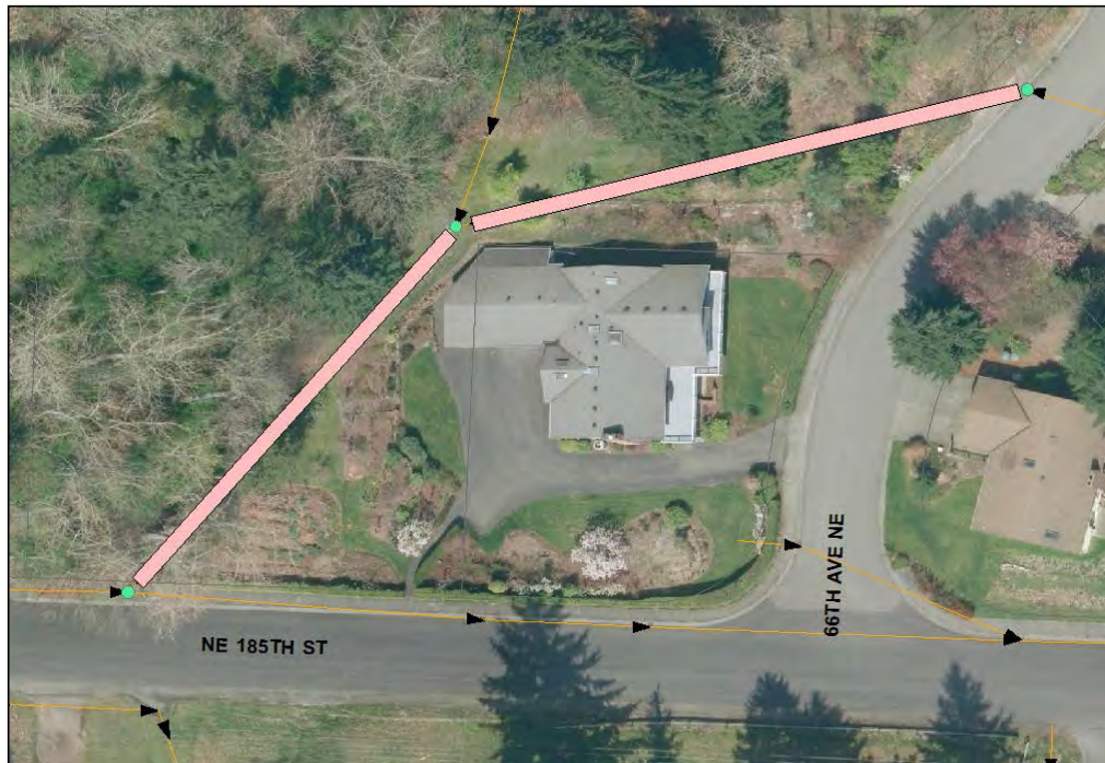
Figure 10: Detention Pipes along NE 185 th Street
