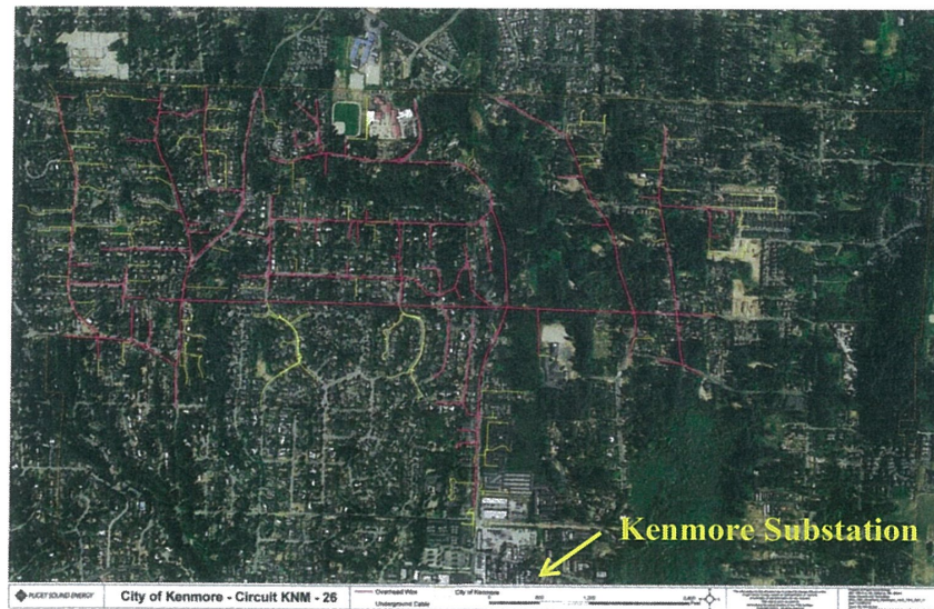
Figure 10. Feeder circuit Kenmore 26; red color is overhead lines and yellow color is underground cables
