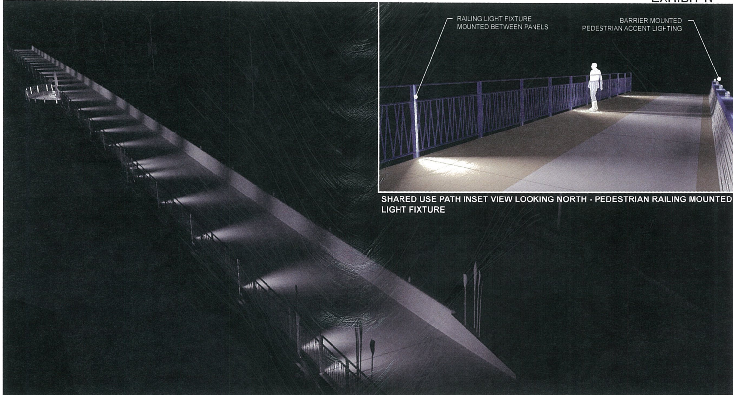
SHARED USE PATH PEDESTRIAN RAILING MOUNTED LIGHT FIXTURE AERIAL VIEW LOOKING NORTHEAST FROM SOUTH ABUTMENT AT NIGHT SHOWING CONCEPTUAL LIGHT LEVELS ONLY.
