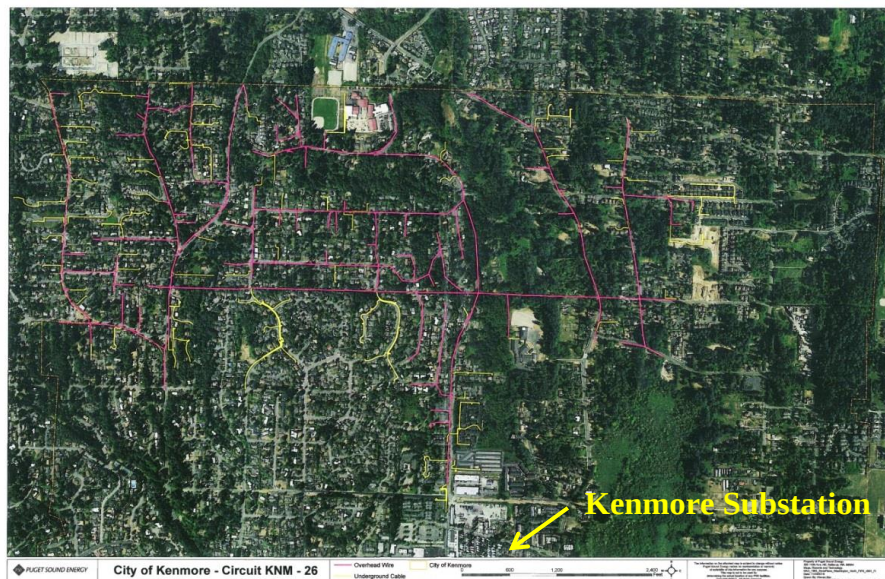
Figure 9. Feeder circuit Kenmore 26; red color is overhead lines and yellow color is underground cables
